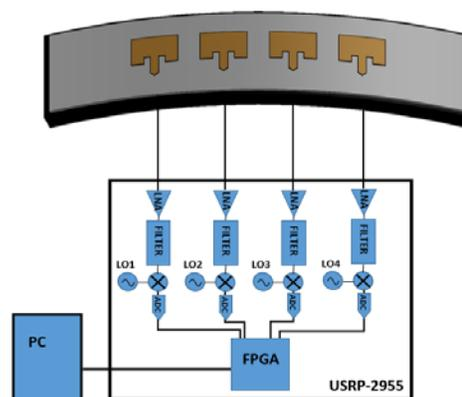
Fig. 1. Conformal antenna array with SDR beamforming.
