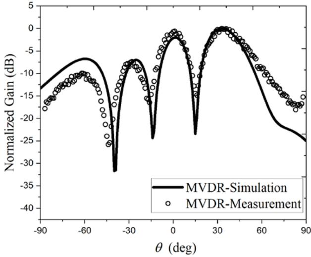
Fig. 3. MVDR normalized radiation pattern with the nulling angle at  $15^\circ$  for desired angle =  $30^\circ$ .
