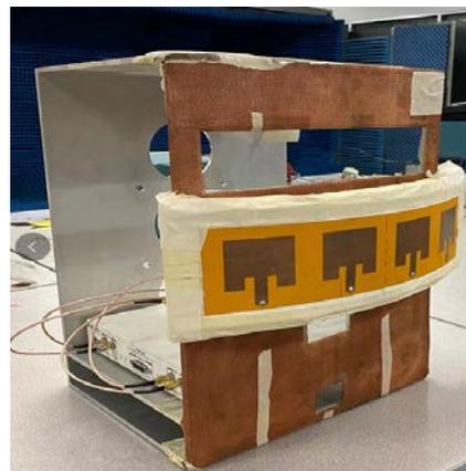
Fig. 2. Set-up of the array on a cylindrical surface with  $r = 733$  mm.
