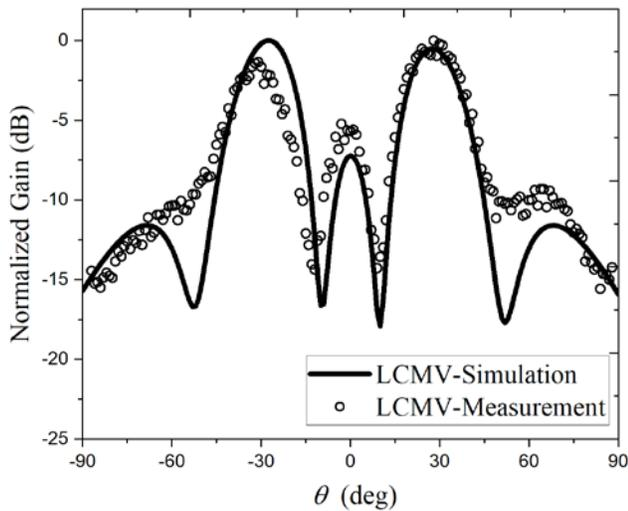
Fig. 4. LCMV normalized radiation pattern with two desired angles at  $\pm 30^\circ$ .
