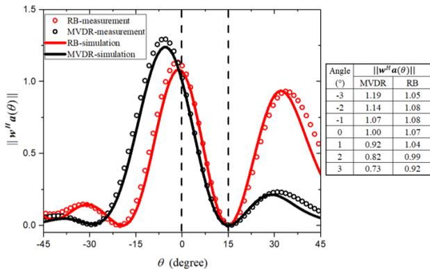
Fig. 5. Simulated and measured array response with a beam at  $0^\circ$  and a null at  $15^\circ$ . The table (right) shows the measured response around  $0^\circ$ .
