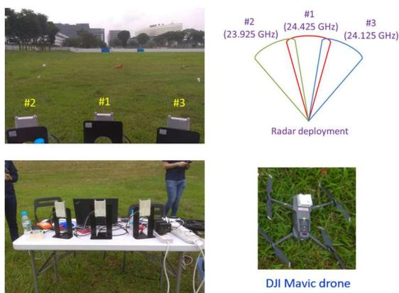
Figure 3: Small radar network and drone trial
