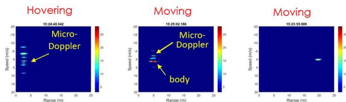
Figure 4: Range-Doppler map with drone detected
