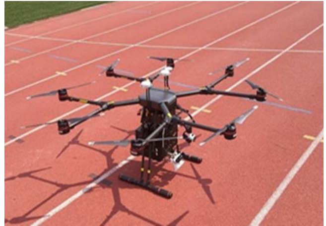
Fig. 1 Integrated Drone SAR System
