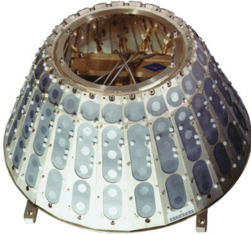
(a) Conical shape satellite antenna, designed to generate three simultaneous and independently steered beams around for data transmission. Alcatel [23].
