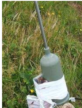
Figure 5.9: HE011 Rohde & Schwarz Aktivantenne
