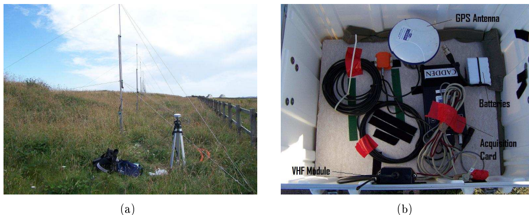
Figure 5.12: (a) Picture of the GPS base near antenna 16 (b) Picture of the GPS module in the hermetic box of the floating antenna.
